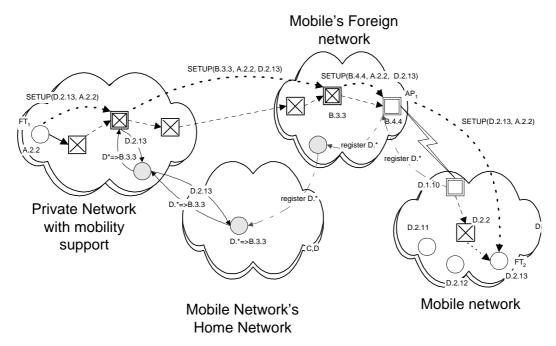
In this example a mobile network is supported. There are assumed to be terminals which are fixed with respect to the mobile network. In this case the Location Service can manage the mobile network as a whole. All endpoints within the mobile network have the same network prefix D which identifies them as mobile. Non mobile-enabled switches will by default route connections to the 'Home Network' of D which is C.
