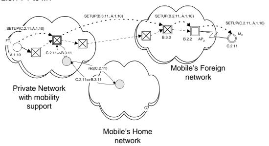
In this example it is assumed that the intervening network cannot support explicit tunnelling. This would be the case for UNI 3.0 / 3.1 networks which have no mechanism for encapsulation of the MHA. Implicit tunnelling requires the MHA and MFA to have a one-to-one mapping. This can be achieved by including the ESI of the MHA in the MFA with the assumption that the mobile ESI is unique.
