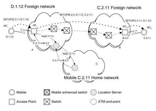
In this example a connection is originated from calling mobile MT<sub>1</sub> and destined for mobile MT<sub>2</sub>. The mobiles themselves only use their respective MHAs, MHA<sub>1</sub> D.1.12 and MHA<sub>2</sub> C.2.11. Access points are assumed to have Location Service functionality and in this case no mobile-enabled switches are necessary. There are no changes to the signalling protocols.
