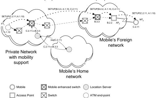
In this example, a connection is originated by  $FT_1$  with ATM endpoint address A.1.10 for mobile  $MT_2$  with MHA C.2.11. The source network is mobile-enabled and the mobile is supported by an anchor switch in its Foreign Network. When the mobile was initially registered at  $AP_2$  the VLR allocated MFA B.3.3 as the anchor switch for the mobile.
