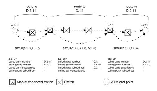
Figure 1: Example of simple tunnelling
