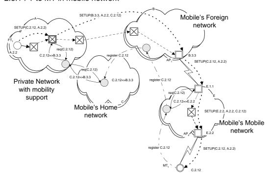
This case is similar to that of a mobile ATM network. In this case the mobile network itself has access points and supports the registration of mobiles. The registration process is hierarchical. Mobile  $MT_2$  registers with the access point  $AP_2$  which itself is part of the mobile network E.
